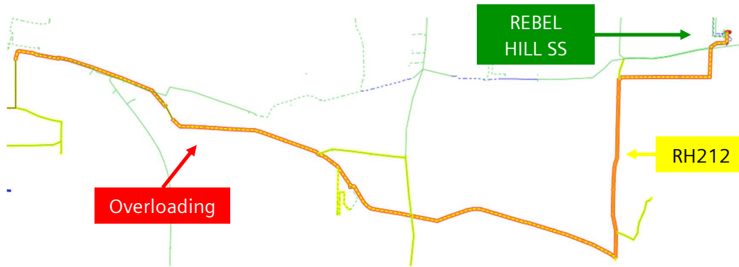
Figure 5-82 Overloading violation under GS232 emergency condition in 2025
